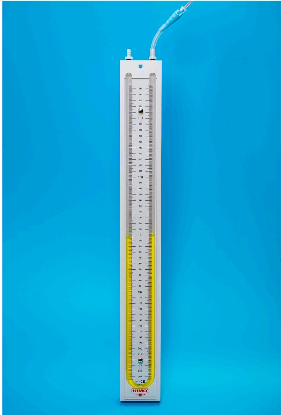
**Figure 4.** U-tube manometer used to measure true intra-cuff pressure. The U-tube manometer was connected via a ridged extension line to the rest of the benchtop setup.
